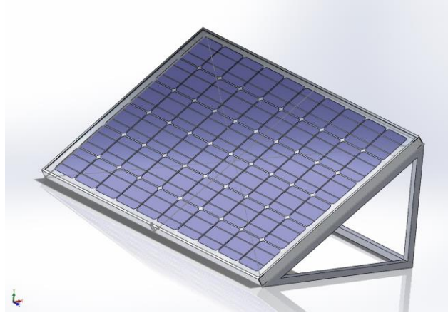
Figure 3.1: Solar panel angled at 35°
