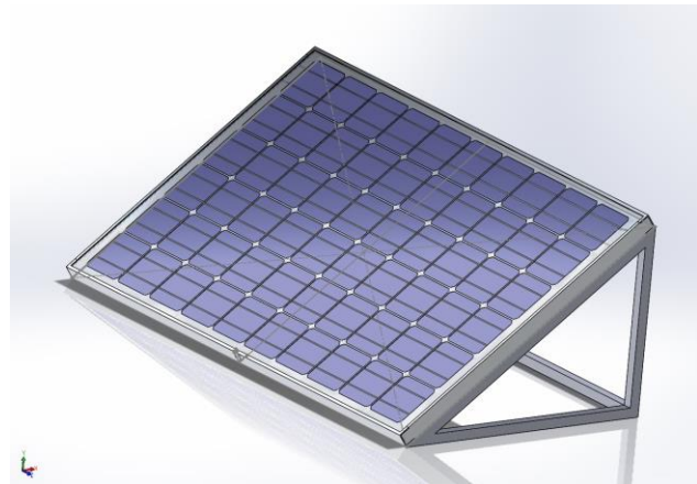
Figure 1- solar panel angled at 35°
