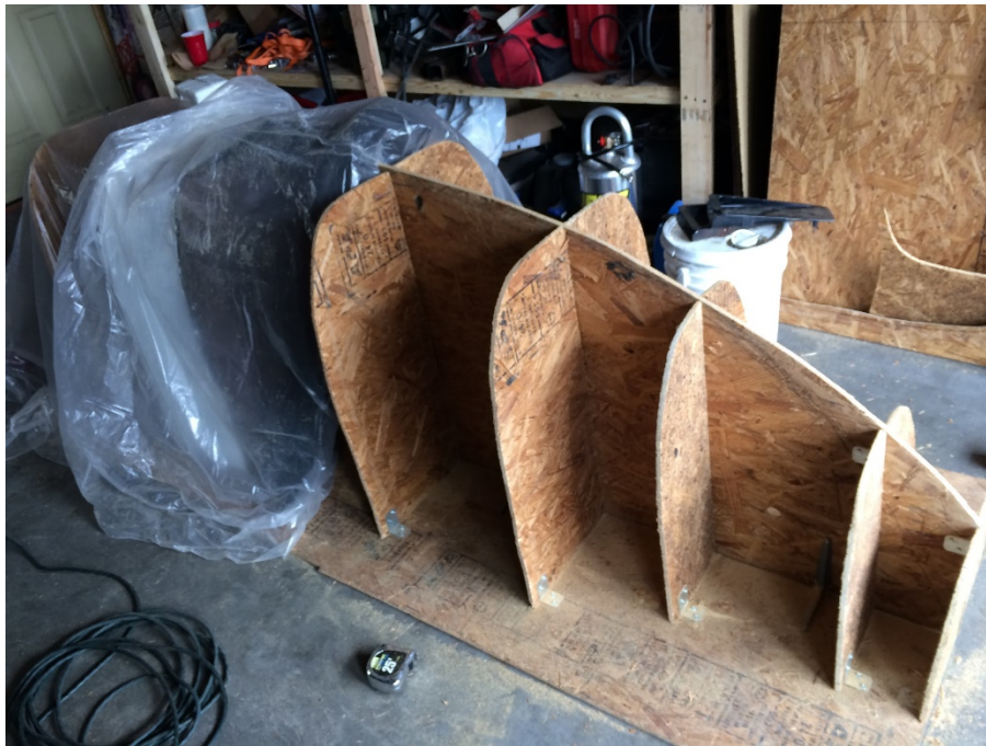
Figure 4.3: Fairing with OSB Sections
