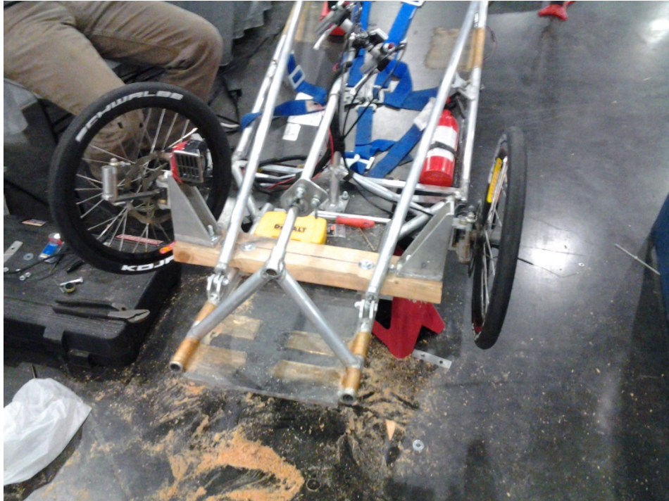
Figure 5.2: Wooden Steering Cross Member
