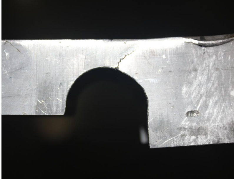
Figure 5.1: Aluminum Cross Member Failure
