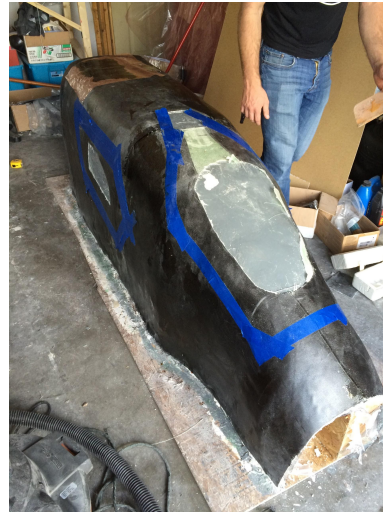
Figure 6: Layup of the fairing on the plug
