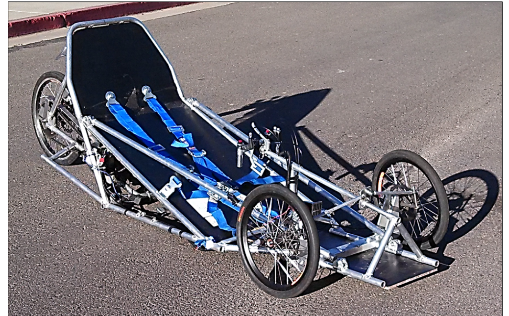
Figure 4: Finished Frame with Other Components Installed
