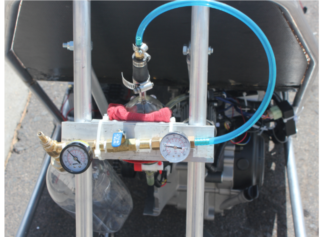
Figure 9: Fuel Pressure System
