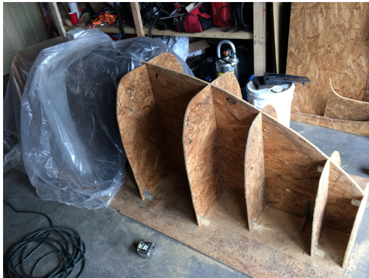
Figure 5: Sections and central spine of the fairing plug.
