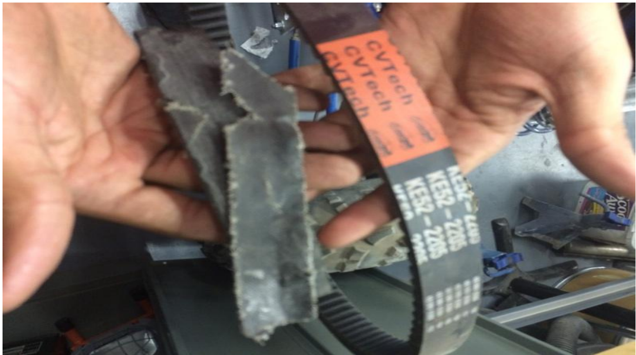
Figure 6C - Old CVT belt (what's left of it) vs. new CVT belt right side
