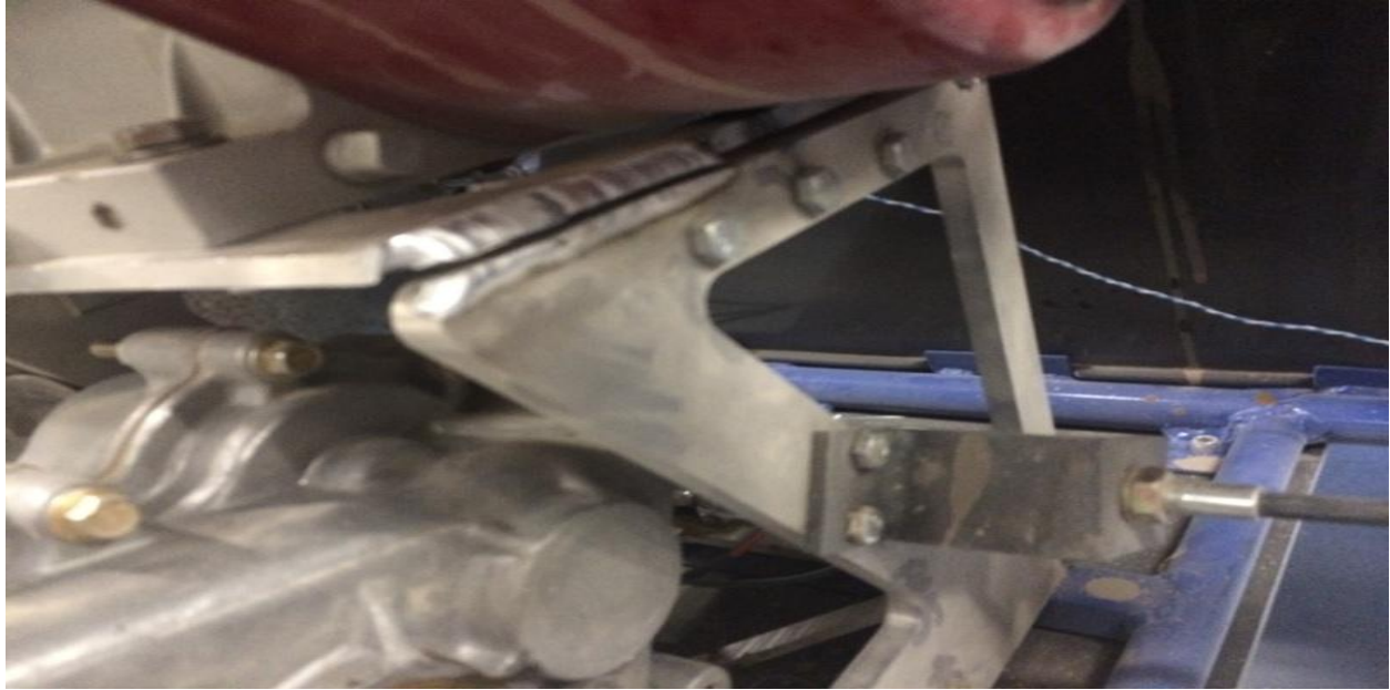
Figure 5C - Broken engine mount
