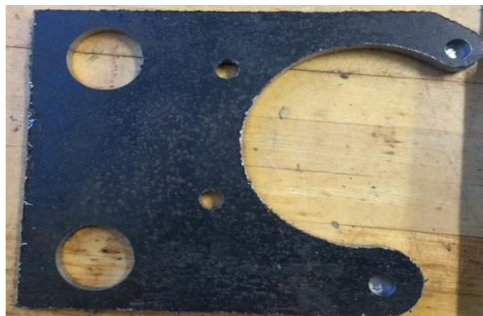
Figure 4.2- CNC cutout of the rear suspension plate
