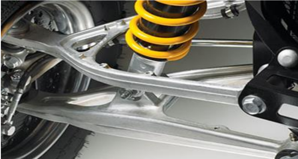
Figure 3 - Double A-Arm suspension [4]
