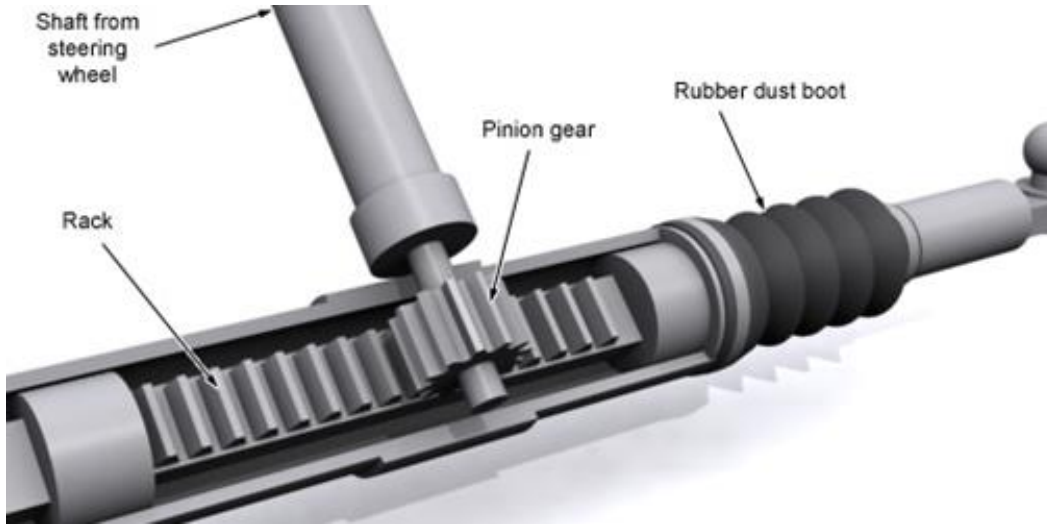
Figure 6: Simple Rack and Pinion with Spur Gear [7]
