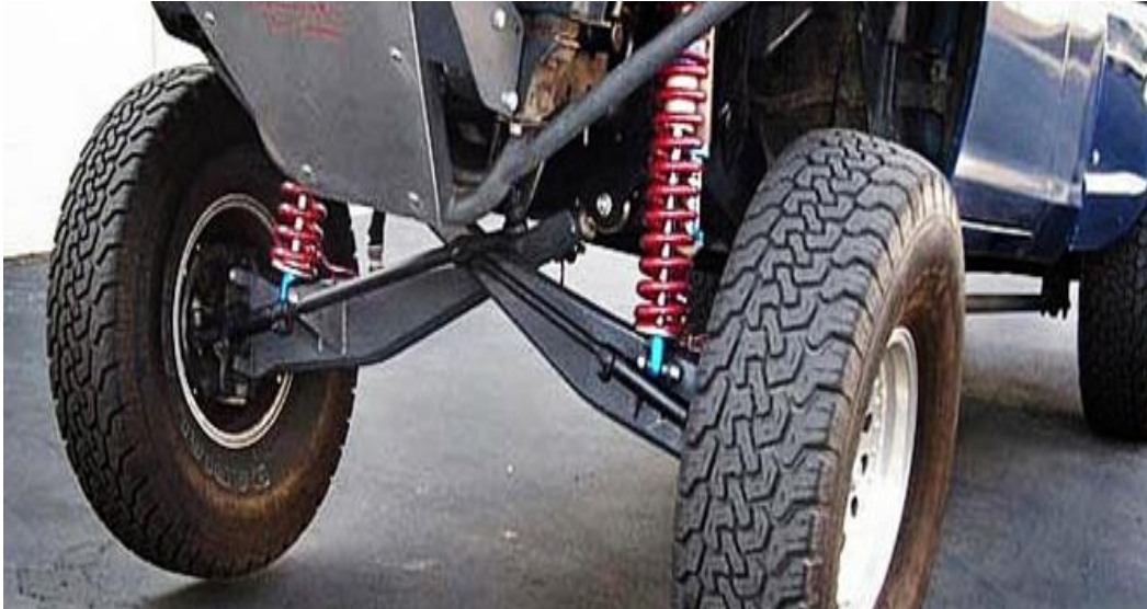
Figure 2 - Twin I-beam front suspension [3]
