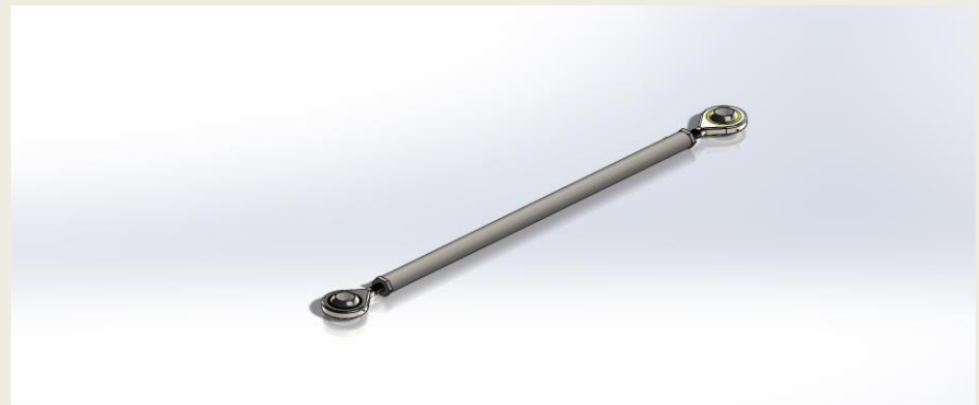
Figure 18: CAD Tie Rod
