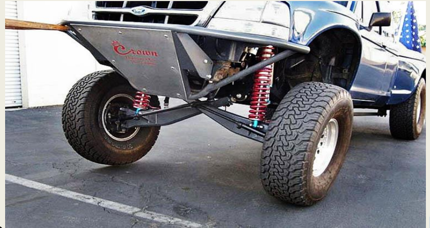
Figure 5: I-Beams Source: HM Racing Design
