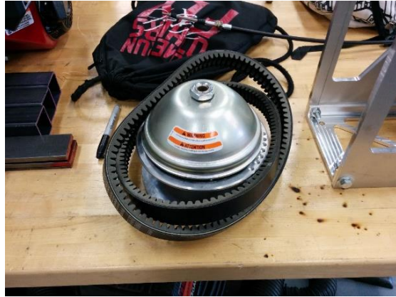
Figure 2: CVT Input Pulley and Belt
