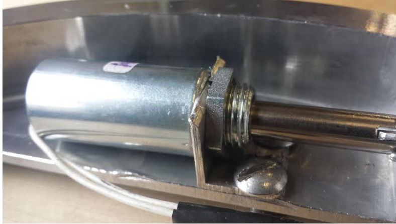
Figure 9: Solenoid mounted onto RR base plate
