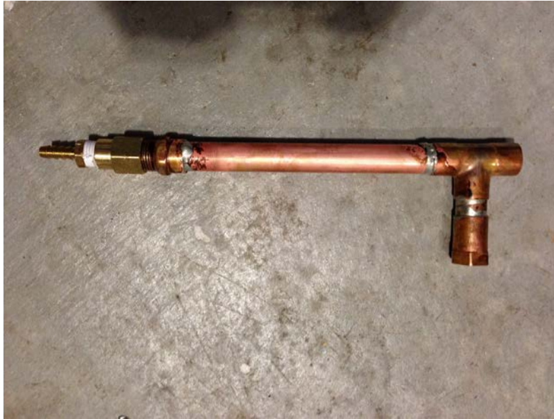
Figure 2.3.1- Inlet/Astrometric hut tee fitting.
