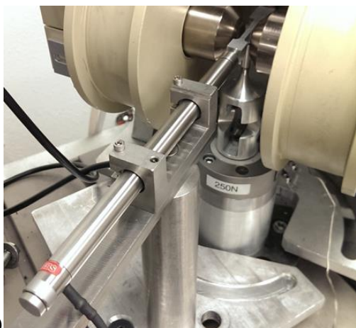
Figure 2.8: (A) Assembled Actuator Mounting System (B) Micro-Tip and MSMA Contact
