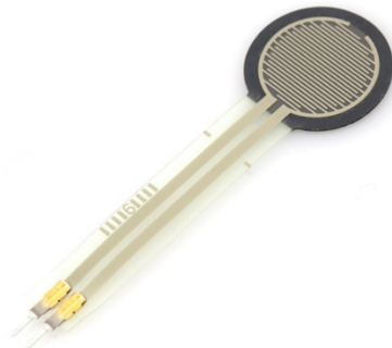
Figure 2.4: General FSR Used to Sense Forces [8]
