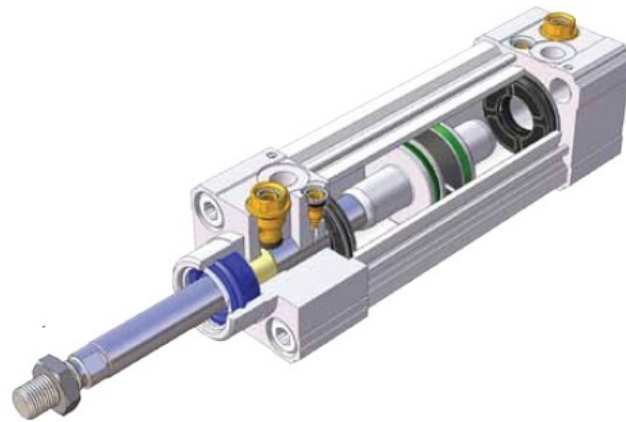
Figure 2.6: General Pneumatic Actuator [3]
