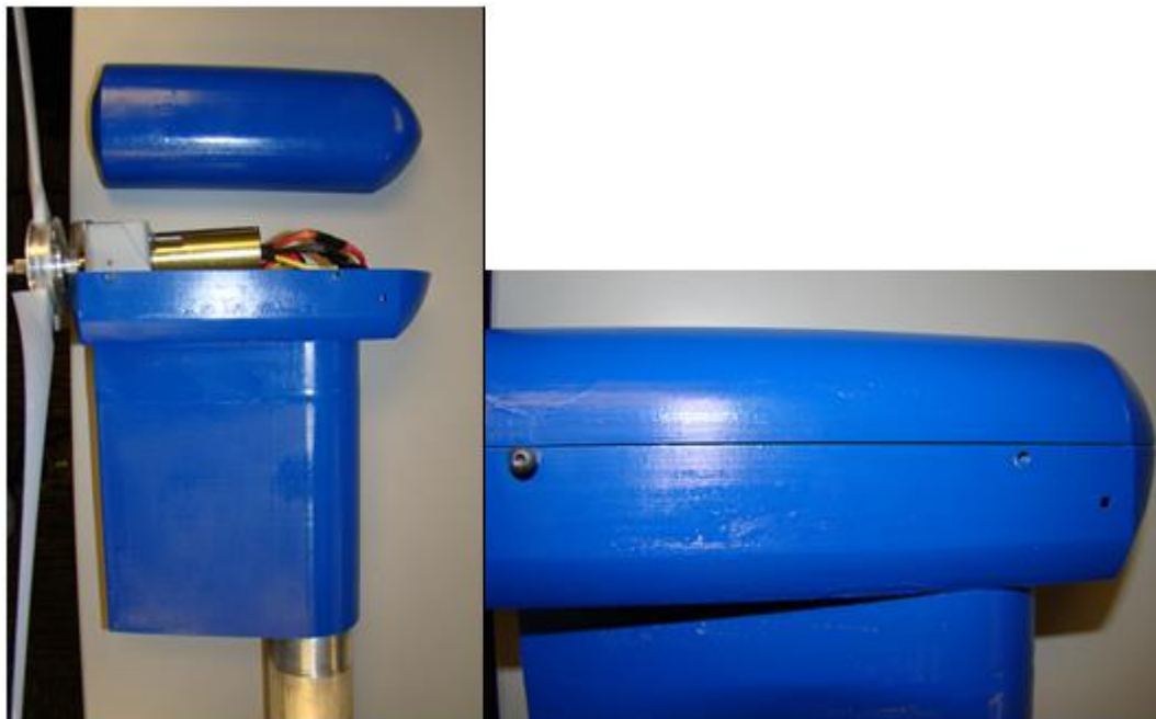
Figure 5: Main Frame and Nacelle Assembly
