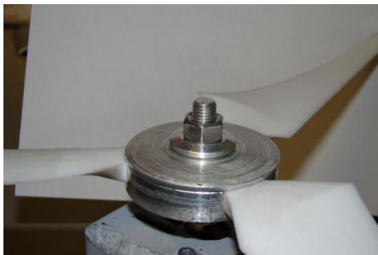
Figure 2: Blade and Hub Assembly
