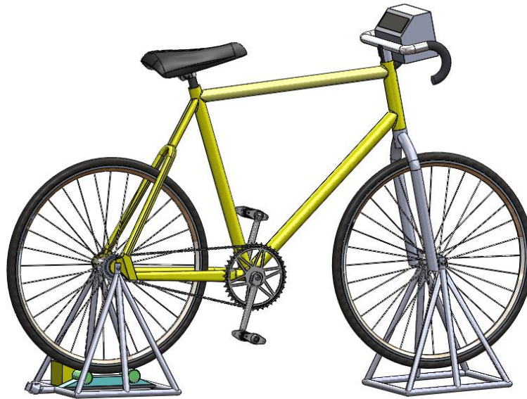
Figure 2 - Charging station (stationary position)
