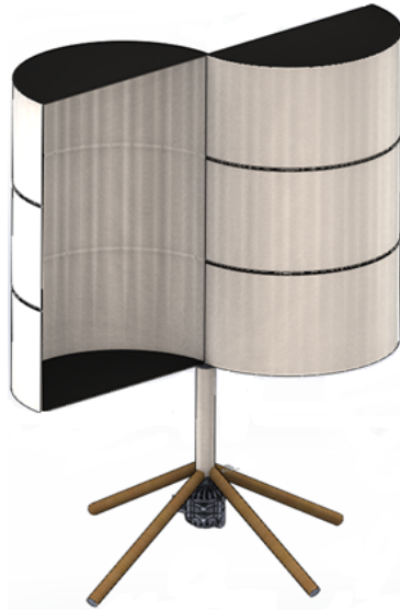
Figure 9: 55 Gallon Drum Turbine
