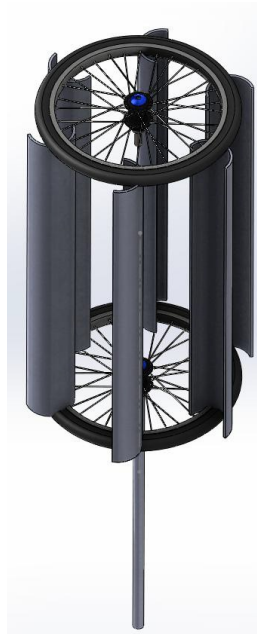
Figure 1 – Final Concept Design, Vertical Bike Wheel Turbine
