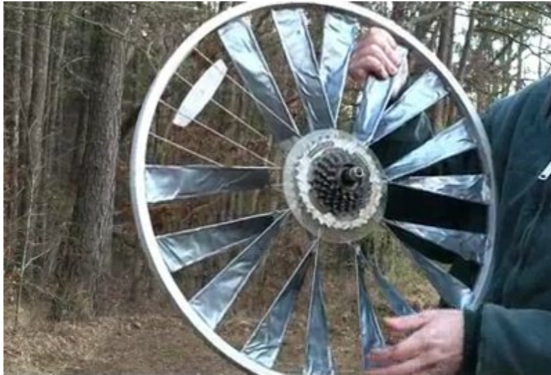
Figure 2 – Final Design Concept, Horizontal Bike Wheel Turbine [1]
