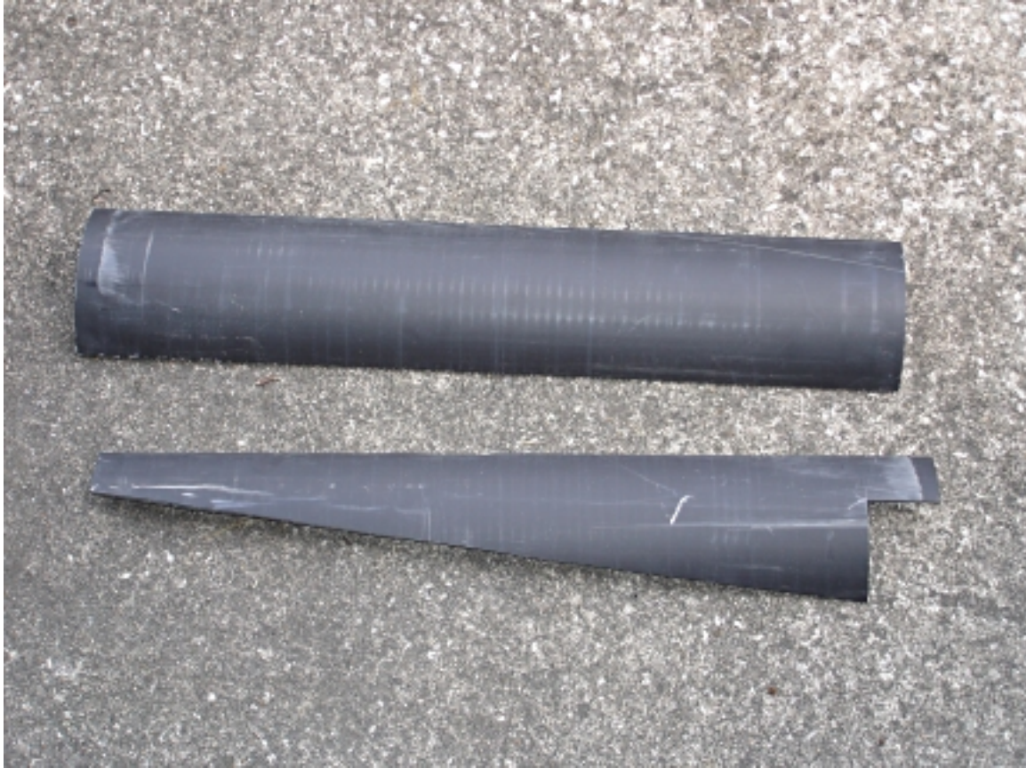
Figure 1 – PVC Turbine Blades [1]
