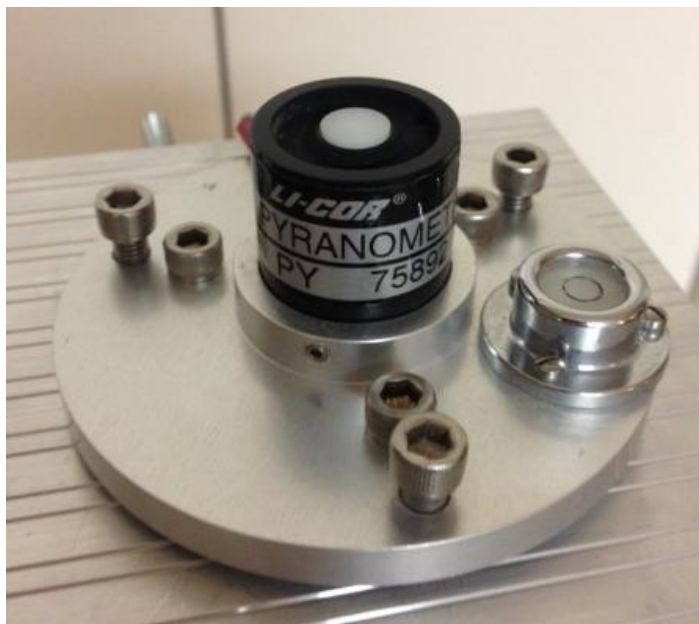
Figure 3. Close-up View of the LI-2003S Leveling Plate
