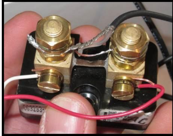
Figure 12. Temporary Shunt Resistor of 1 ohm.
