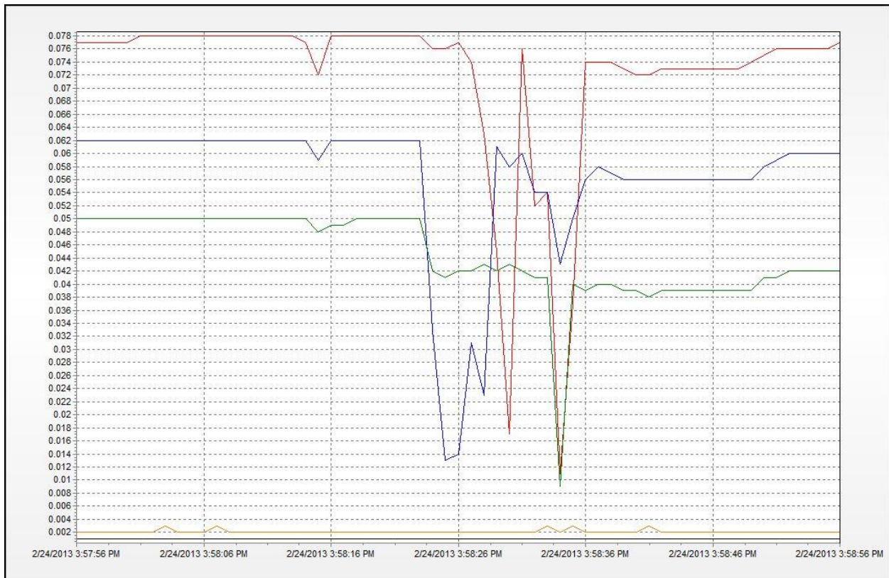
Figure 11. Pyranometer Voltage Outputs at 1Hz (left axis is mV).
