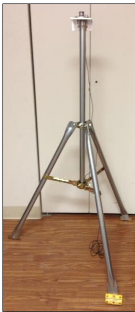
Figure 7: Tripod with pyranometer mounted
