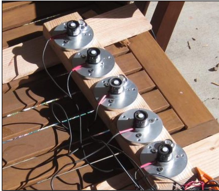
Figure 3: Pyranometer calibration setup
