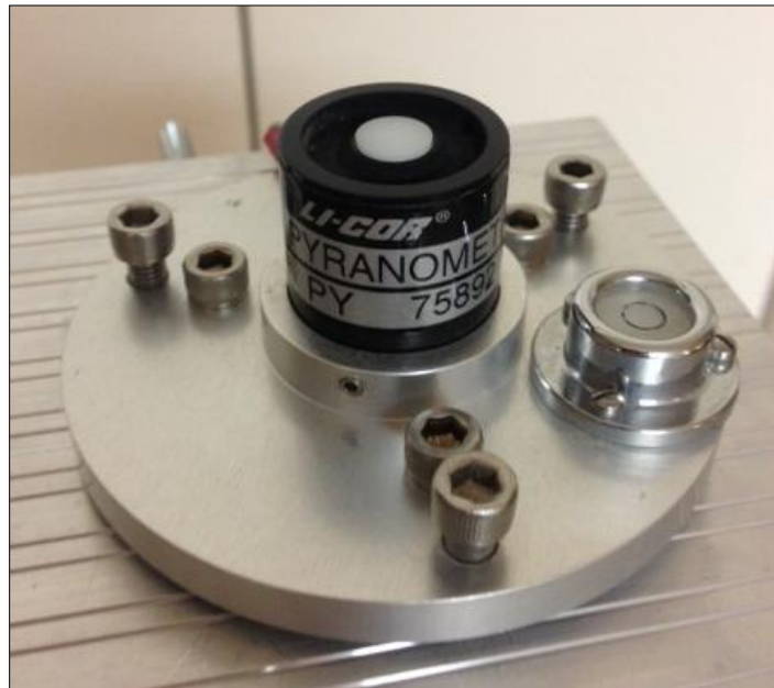
Figure 5: Close-up view of the LI-2003S leveling plate
