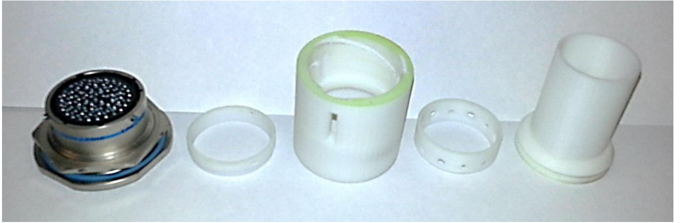
Figure 3: Exploded view of first FDM prototype
