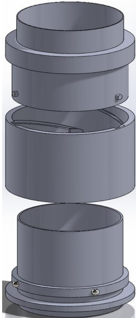
Figure 5: Modified ball bearing detent design (exploded view)
