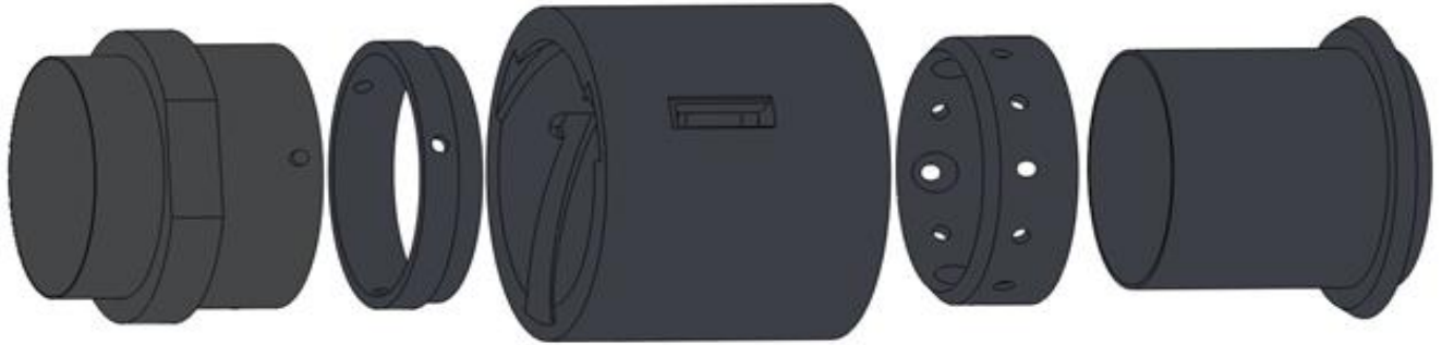
Figure 13: Ball Bearing Detent: Exploded View
