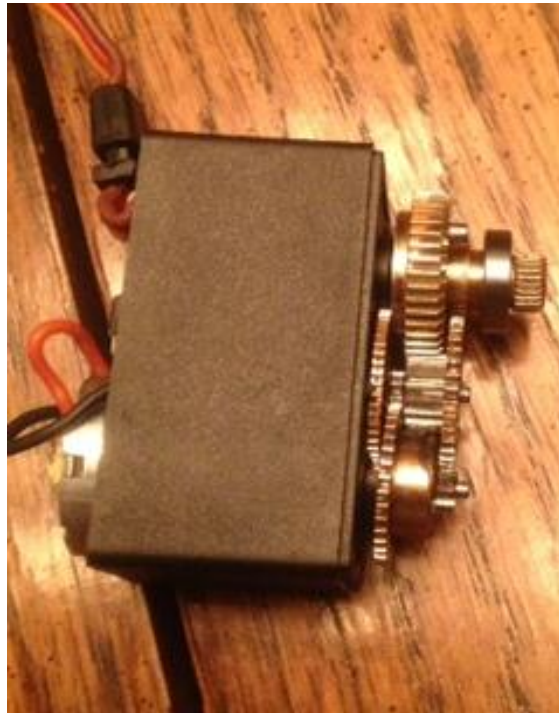
Figure 12: Gears of a Servo
