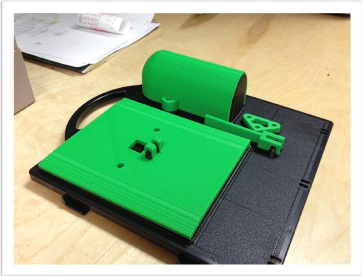
Figure 14: All four pieces after being made using the FDM
