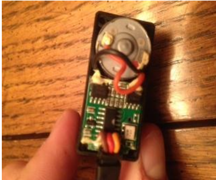
Figure 11: Computer and motor components of a servo
