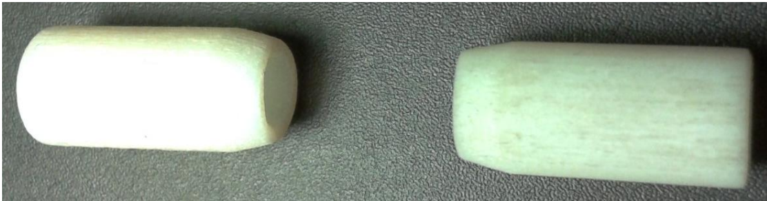
Figure 2 – The left sleeve has tighter tolerances than the right sleeve
