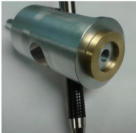
**Figure 23 – Press fit washer**
