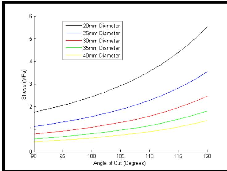
**Figure 26 – Stress vs. Angle**
