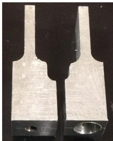
**Figure 19** – Micrometer tips
