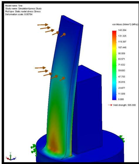
**Figure 27** – SolidWorks Tine Analysis
