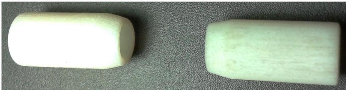
**Figure 12** – The left sleeve has tighter tolerances than the right sleeve
