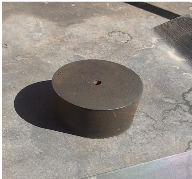
Rubber Stopper Used to Hold Mirror Cover
