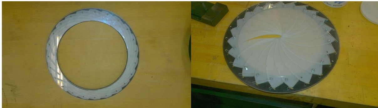
Figure 5 – The Iris prototype version 1.0 in the open position on the left and in the closed position on the right.
