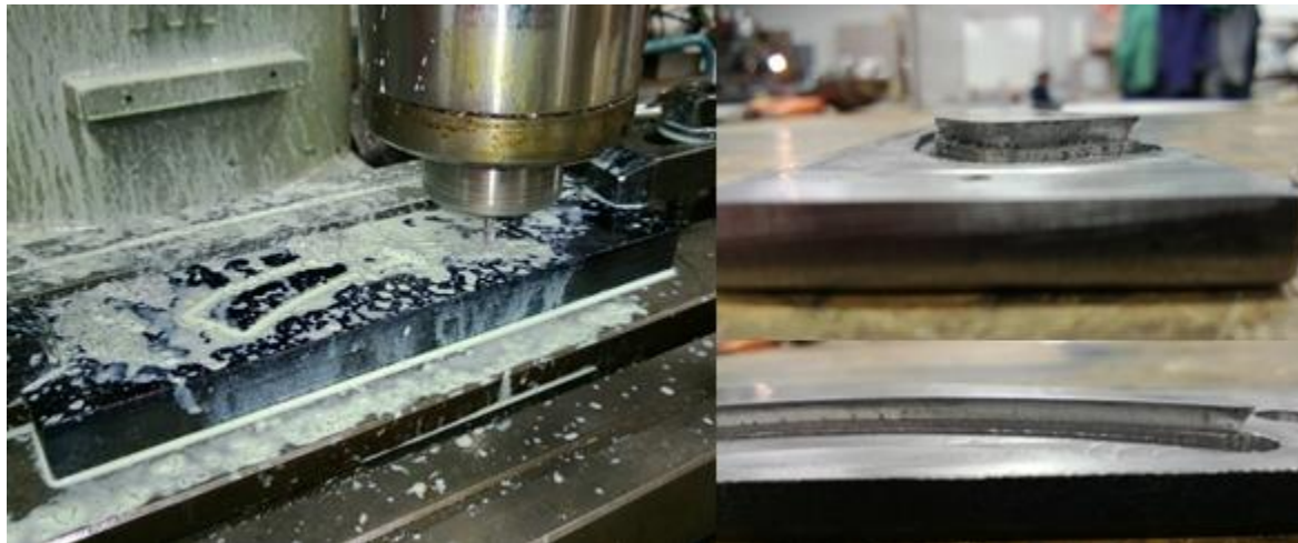
Figure 2 –Stamp Being Machined
