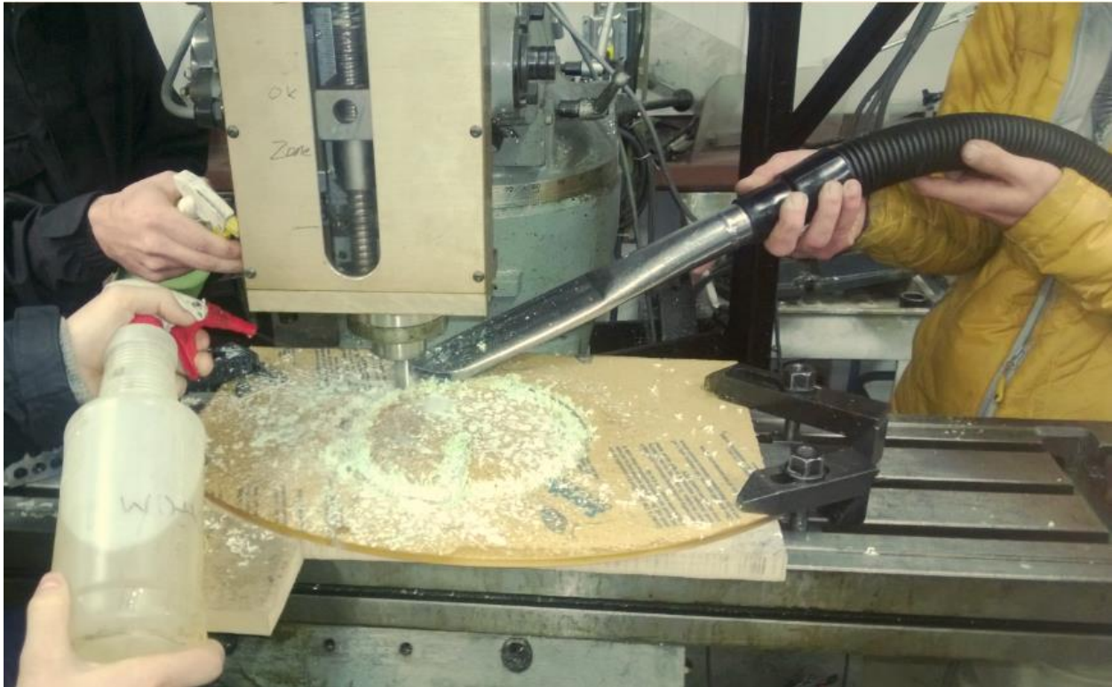
Figure 4 –Iris Rings Being Machined
