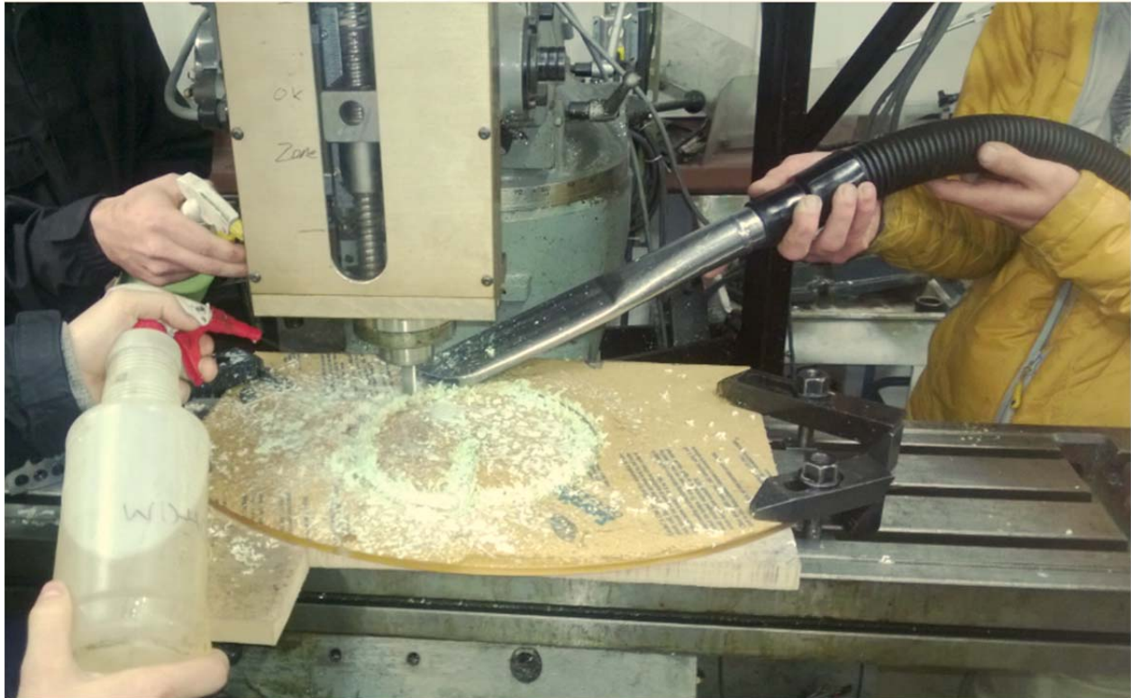
Figure 5 –Iris Rings Being Machined
