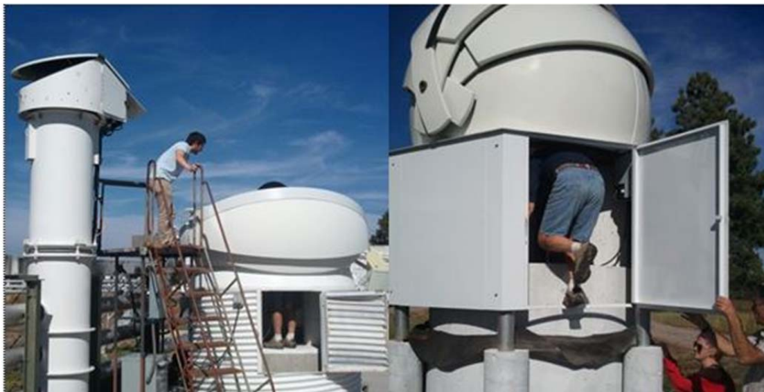
Figure 2-Employees of NPOI must climb into the dome housings in order to manually remove the mirror cover.
