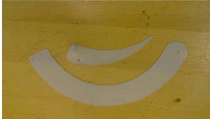
Figure 4 – The initial Iris blade compared to the second iteration.
