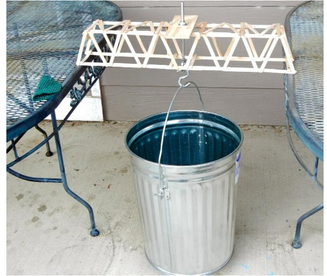
Figure 22: Simple load test typically used for bridge design. [20]
