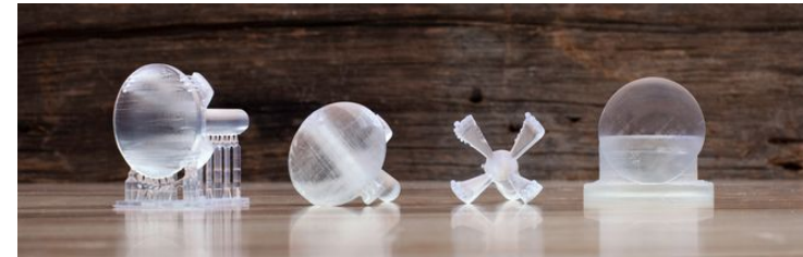
Figure 10: Lens Printing Demonstration of the Form 1+ 3D Printer [16]
