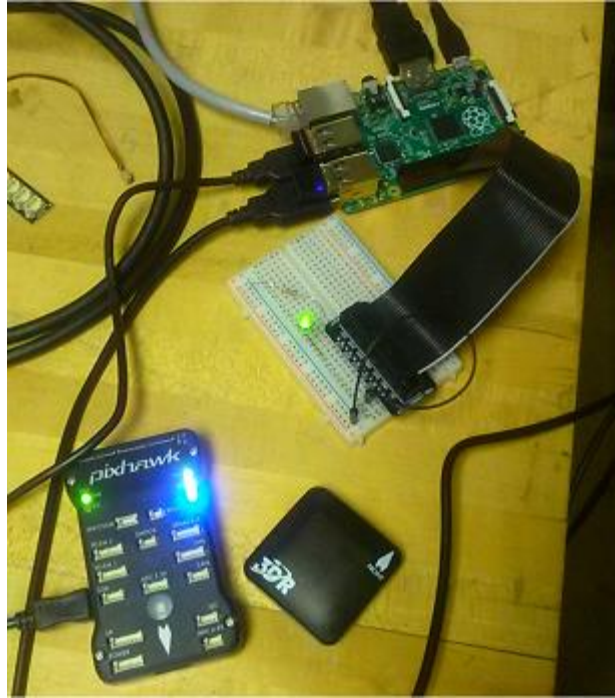
Figure 6. Early prototype demonstrating Pixhawk and RPi function.
