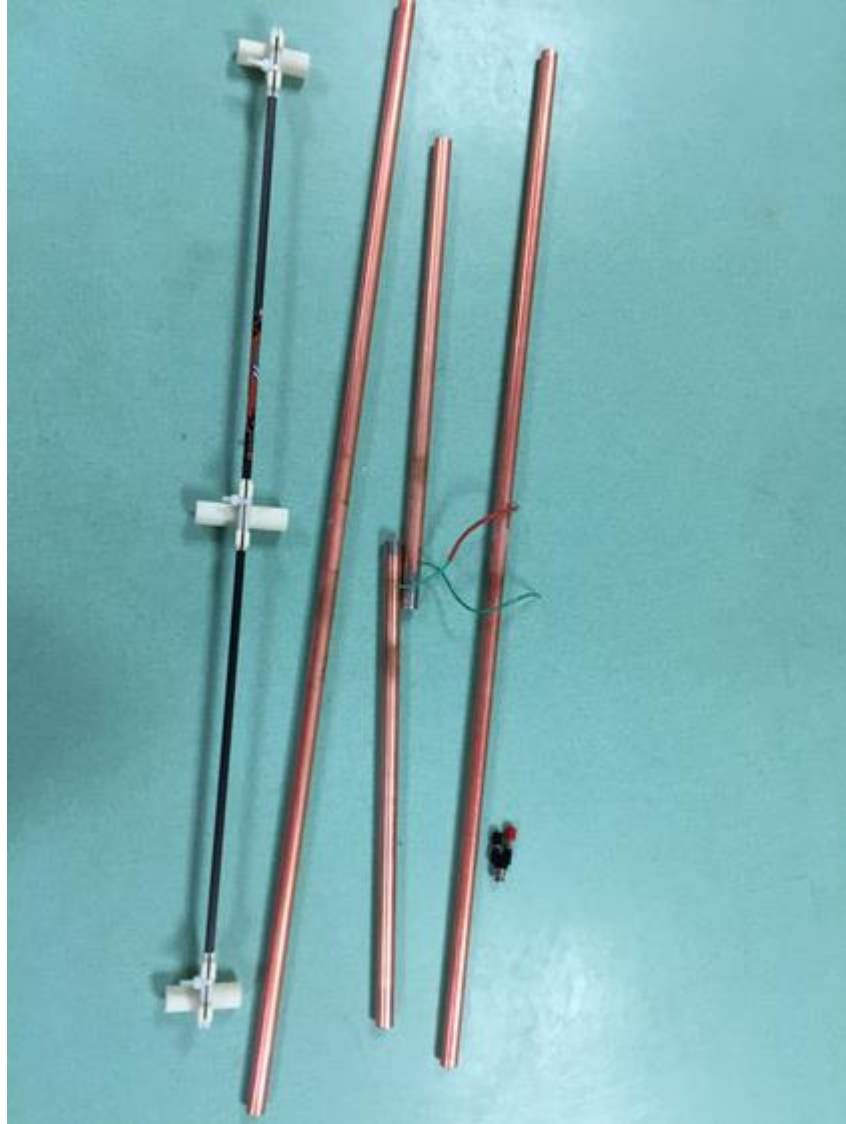
Figure 17. Final antenna in its collapsed, backpackable form.
