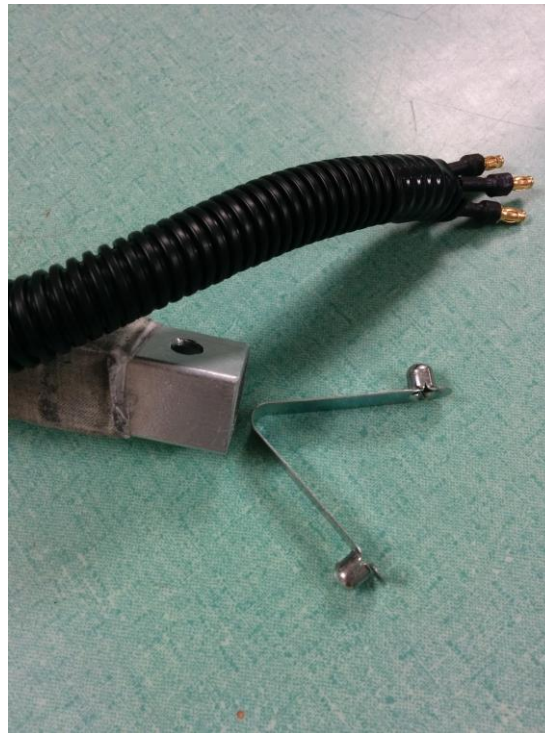
Figure 2. Spring-pin connection for detachable arms.
