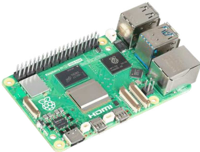
Figure 28 Ball-on-Beam Prototype: Raspberry Pi
