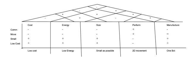
This is the house of quality which was made based on the matrices. The requirements are very vague because at the moment we only have the goals of our robot and so we have to go off our budget of \$500 to get accurate requirements for what we are aiming for.
