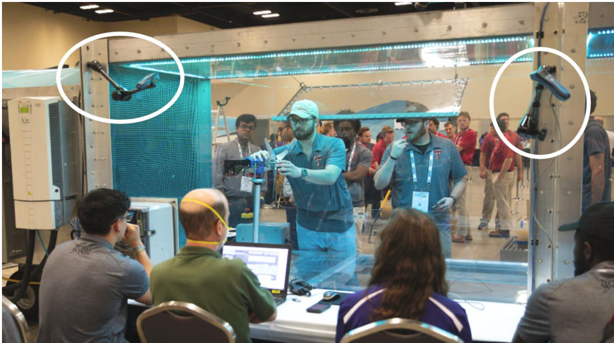
Figure 17. Laser tachometer sensors (circled in white) used to measure turbine RPM.
