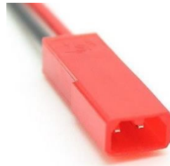
Figure 14. Team-provided connection to the manual shutdown interface
