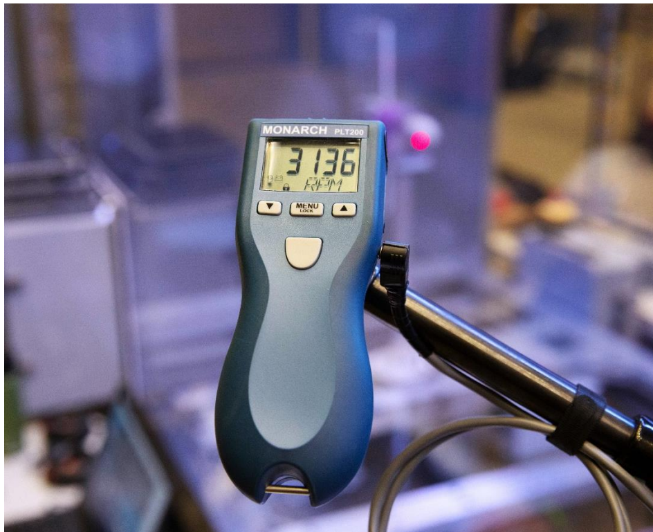
Figure 16. Laser tachometer used to measure turbine revolutions per minute
