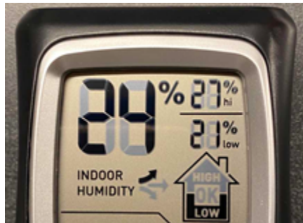
Figure 2A. Commercial thermometer-hygrometer for test comparison.
