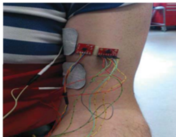
Figure 2: Experimental Setup & accelerometer position (ADXL335)
