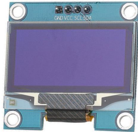
Figure 2: OLED screen taking the place of LCD
