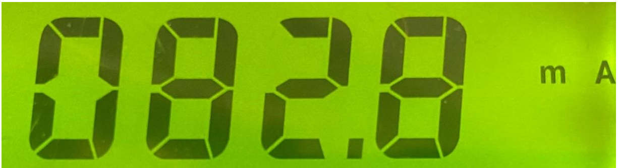
Figure 5: Inspection Test - Current Usage WiFi Modem
