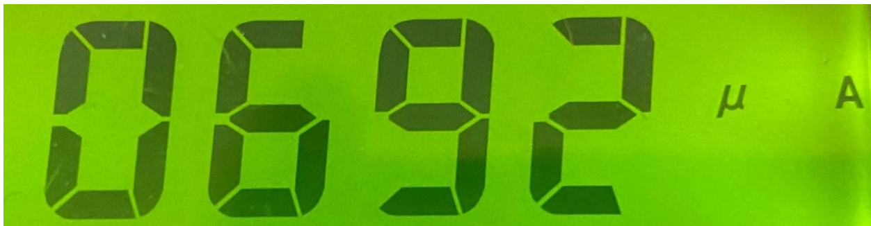
Figure 7: Inspection Test - ESP8266 Deep Sleep Current Usage
