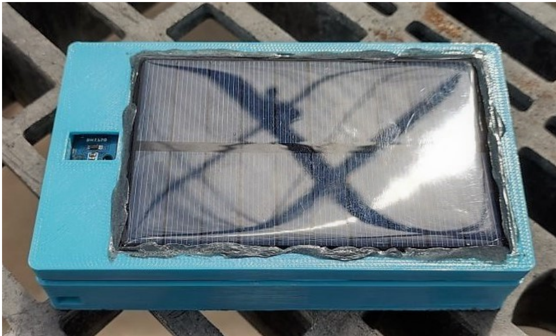
Figure 11: Unit Test - Module Days After Waterproofing Test
