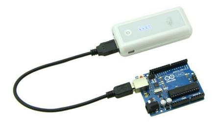
Figure 9 : *Connecting Arduino Uno to a power supply.* 11. Connect the L298 Dual H-bridge with the motors and the 12 V battery.
