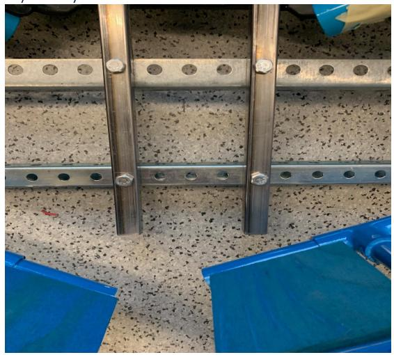
Figure 4 : Drilling on metal bars & attaching them on punched square tube zinc plated.
