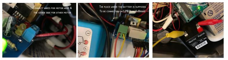
Figure 10: Connection on L298 Dual H-Bridge, Linear Motor wires & battery.
