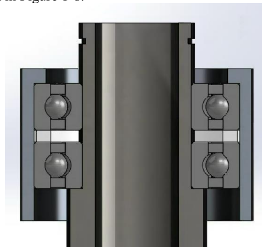
Figure 1-8: Yaw Bearing Assembly
