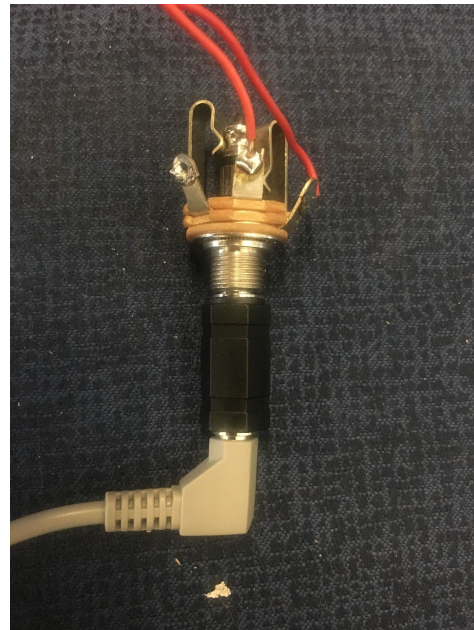
Figure 17: Correct Wire Connection
