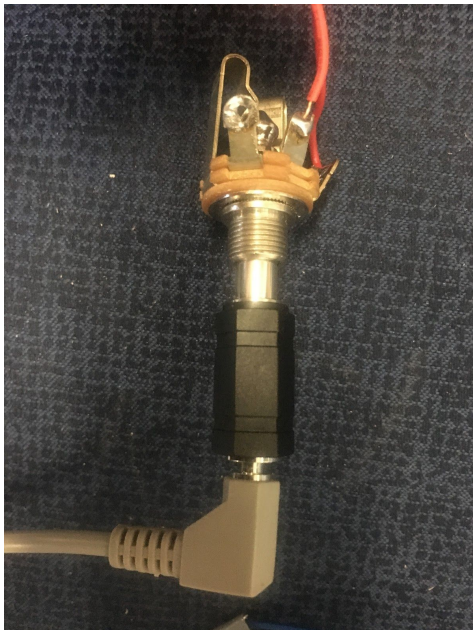
Figure 16: Incorrect Wire Connection
