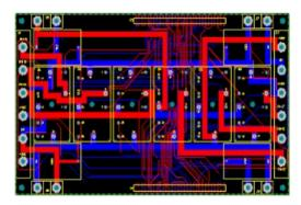
NPC power board converse three phase power into DC using three "SK20MLI066" switches devices every device has 4 IGBTs models. Furthermore, the NPC power board will be reused for three main high power applications.
