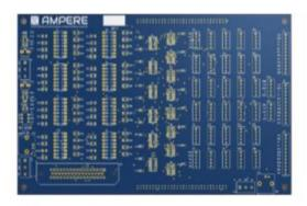
dSPACE Interface Board is used for real time implementation of model predictive control. This will Convert TTL logic signals from the dSPACE DS1103-based to CMOS logic (MC14504 component).
