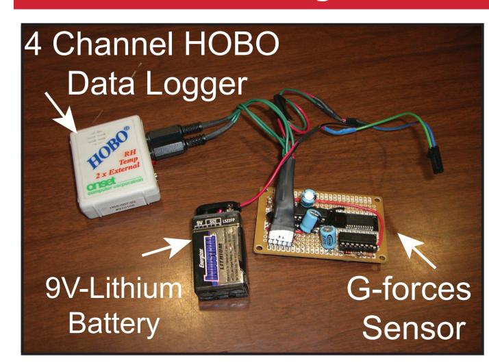
The sensor subsystem includes a digital thermometer to measure internal temperature variations, a pressure sensor, and vertical and horizontal accelerometers to measure flight G-forces. All sensor output data will be stored on two HOBO data loggers.
