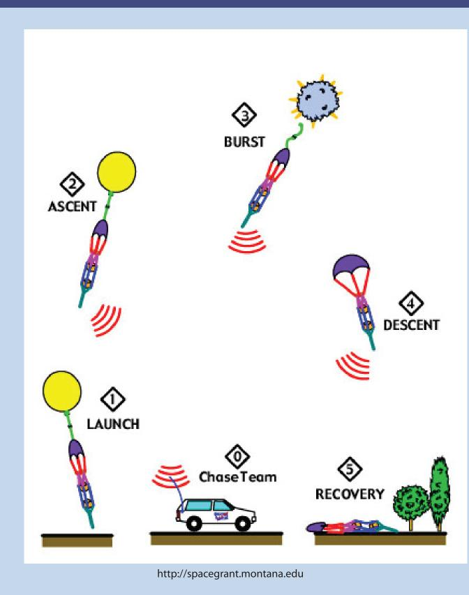
Step 0: The chase team should establish a wireless link with the payload before it is launched. The chase team will follow the payload by following the tracking beacon in the location mapping software.
