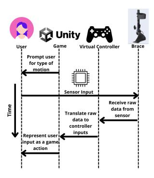
**3.5** User Interaction Workflow for Gamified Rehabilitation: This diagram shows the flow of data from the user's motion to the Unity game interface, via sensor input from the exoskeleton. As the user performs a motion, the sensor captures raw data, which is then translated into game controller inputs that represent the action in the game. This loop provides real-time feedback, enhancing user engagement during rehabilitation exercises.
