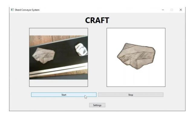
Upon starting our program and placing sherds onto the conveyor belt the camera display screen will start up. When sherds move through the center they will be photographed, an unedited original capture will be saved along side
