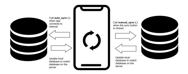
The Home View module will handle the initial synchronization of the application to the API. This synchronization will happen automatically when the application starts. It will send a request to the API to download a recent copy of the main database.
