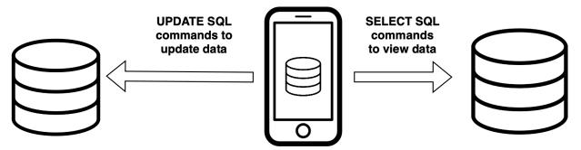
The database that is locally stored on the device will be able to be accessed by the application using an SQLite3 library. This library uses a transaction function to access the data.
