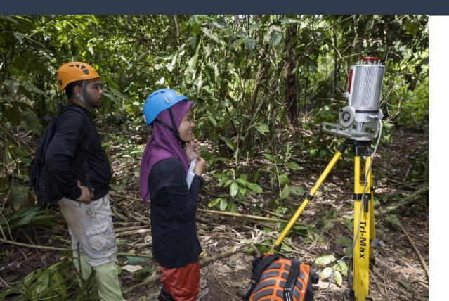
Two members of Dr. Shenkin's research crew scanning the forest using a 360 degree LiDAR on a tripod.
