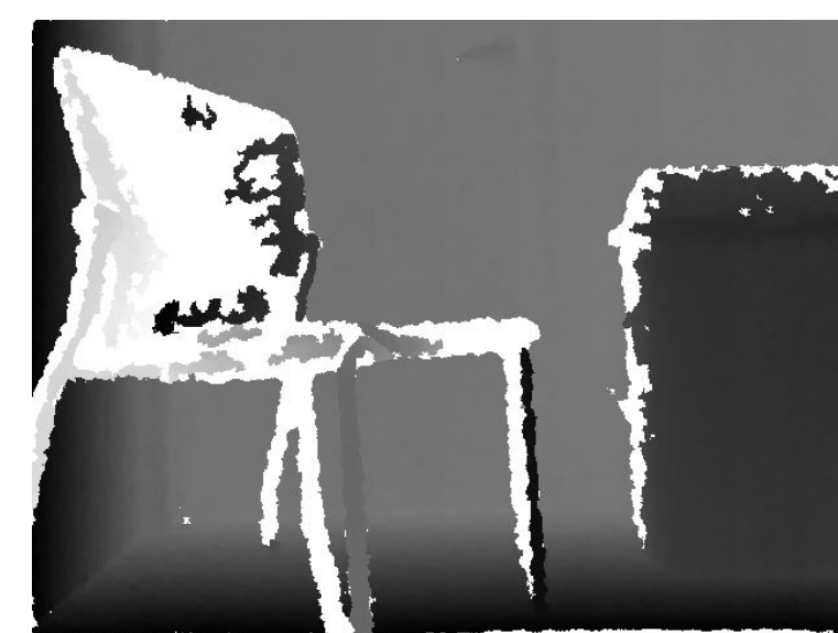
Figure 6 Raw Depth Image from Kinect Sensor
