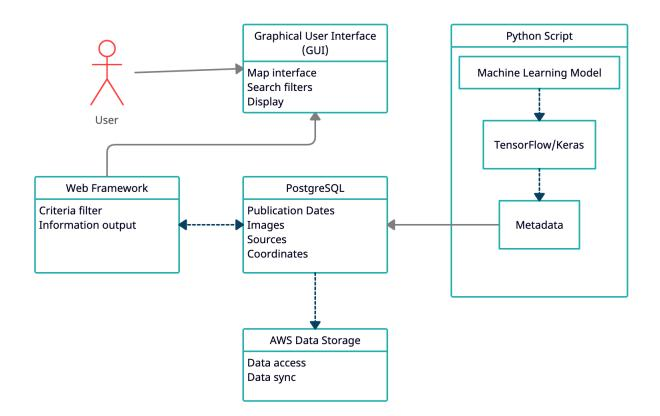
Figure 1. System diagram for MapONE.
