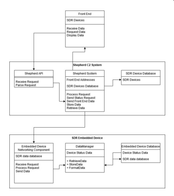
The above diagram details which details our envisioned system architecture and provides some key insights into our project design. Starting from the bottom of the diagram, and moving our way up, the reader can see that the SDR embedded device, or in our case the SDR embedded device being simulated on a Raspberry Pi 3 B+, contains three core components:
