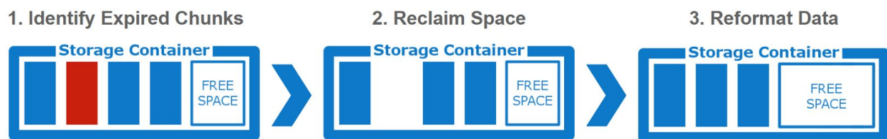
Figure 3: Storage Reclamation Process
